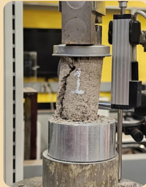
Figure 8 Tensile Failure Mode under UCS
